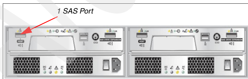
Figure 3-5 DS3200 RAID controller with one SAS host port
